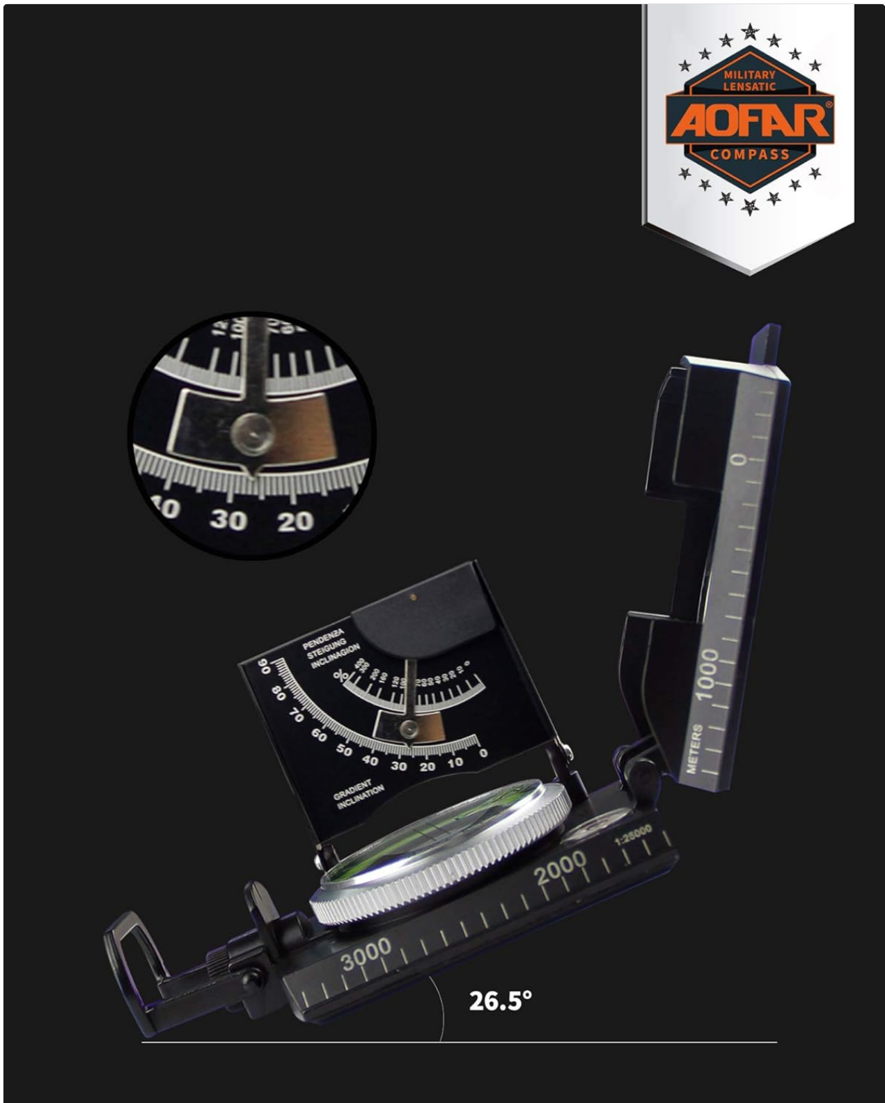
Figure 4.3: The inclinometer allows for measurement of slopes and elevations.
