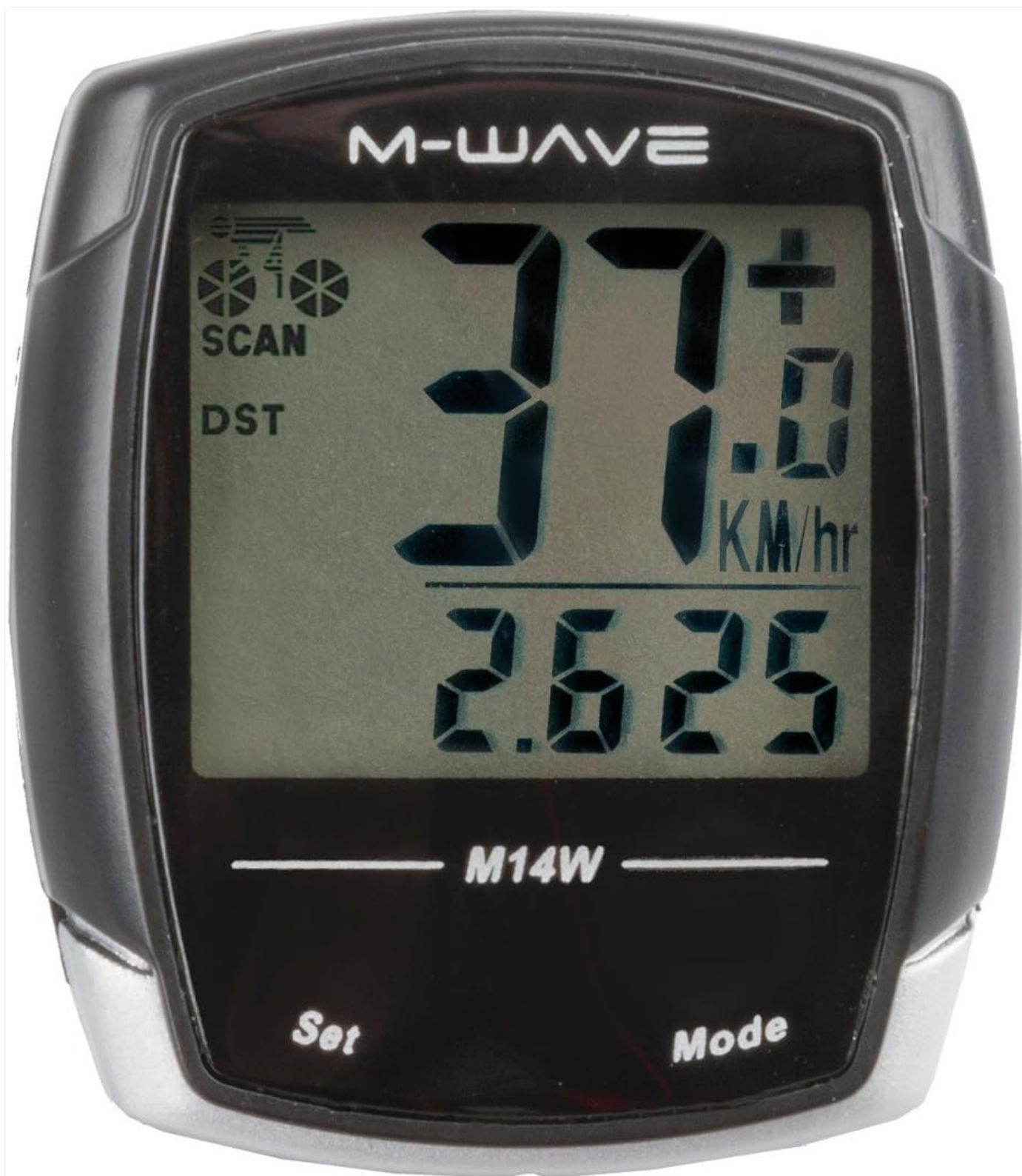
Image 1.1: Front view of the M-Wave M14w bicycle computer displaying speed and distance.
