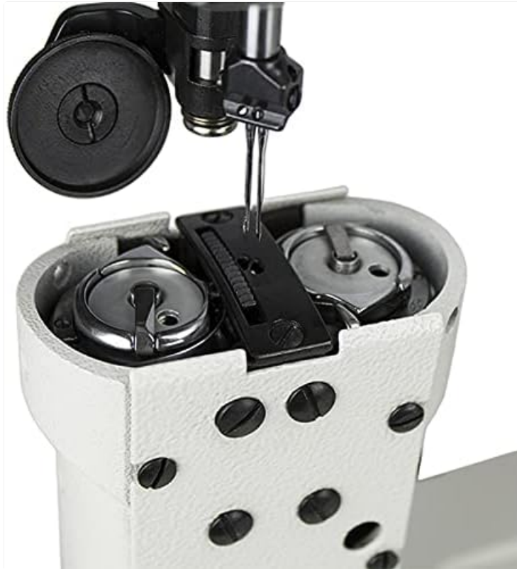
Figure 4.2: Close-up of Sister Speedway SW-820 Double Bobbin Area. A detailed view of the double bobbin and shuttle hook area located within the post-bed of the SW-820 machine. This design allows for two independent lower threads, essential for double-needle stitching. The bobbins are easily accessible for winding and replacement.
