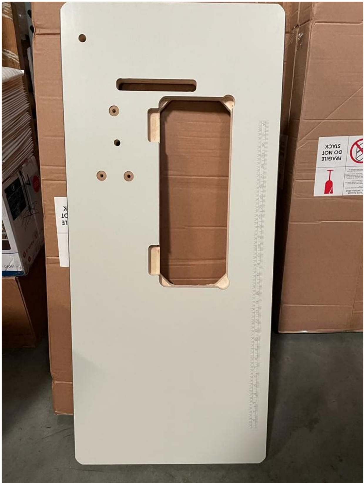
Figure 3.3: Industrial Sewing Machine Tabletop. A view of the industrial sewing machine tabletop, featuring pre-drilled holes for mounting the machine head and other accessories. It includes a cutout for the machine's post-bed and a ruler marking along one edge for convenient measurement during sewing.
