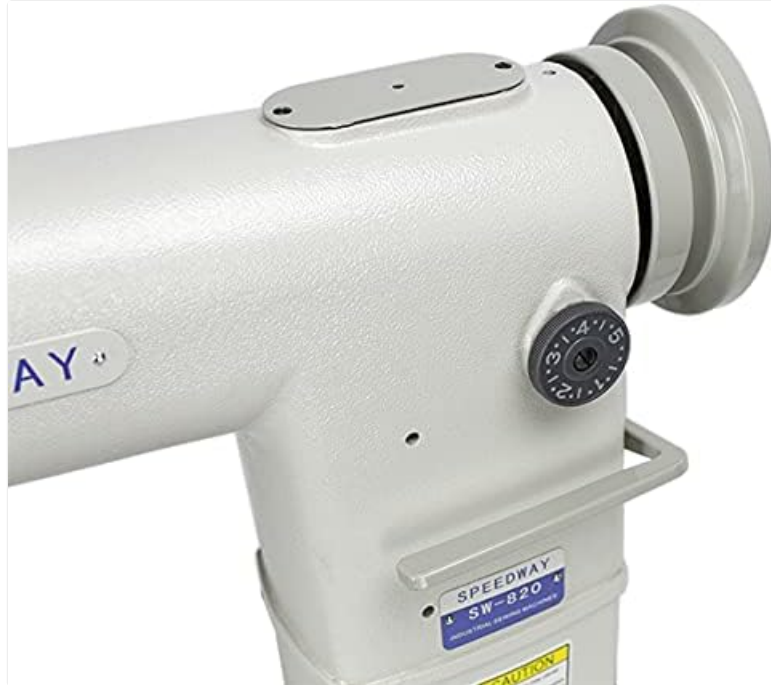
Figure 4.4: Sister Speedway SW-820 Stitch Length Adjustment Dial. This close-up shows the stitch length adjustment dial located on the machine arm. The dial is clearly marked with numerical settings, allowing the operator to precisely select stitch lengths from 0 to 4mm for various material thicknesses and desired stitch patterns.
