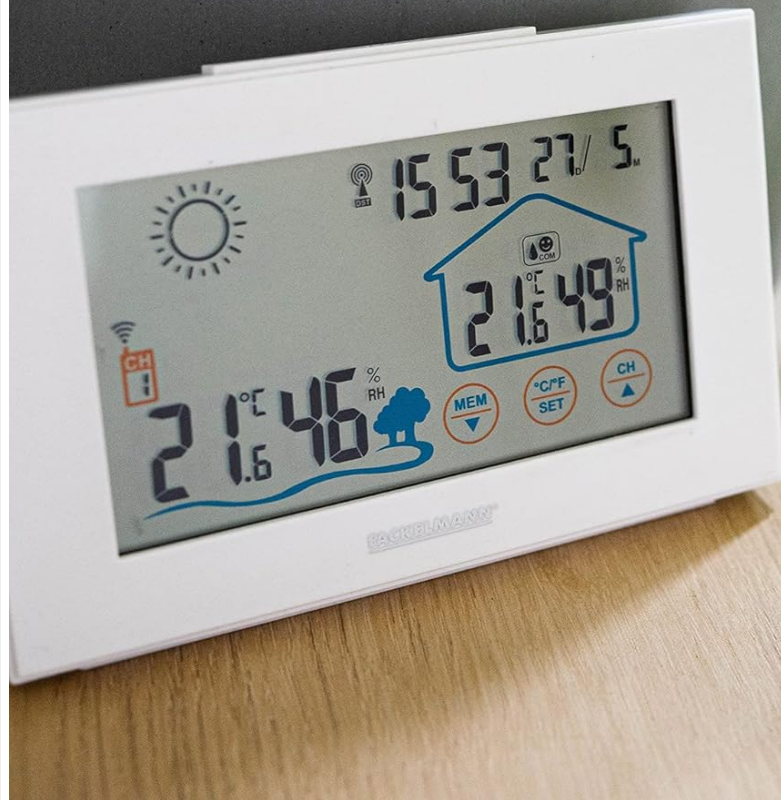
Figure 3: The main unit display showing time, date, indoor/outdoor temperature and humidity, and weather forecast symbols.
