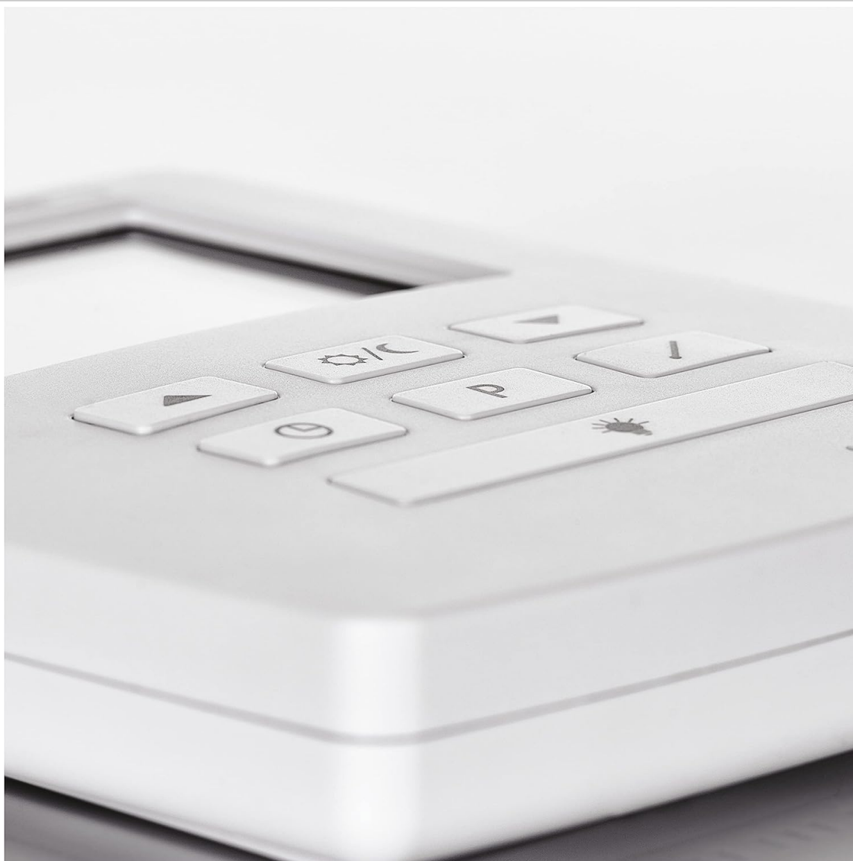
Image 5.2: Close-up of the control buttons on the EMOS P5611OT, including navigation arrows, program (P), and mode (O/C) buttons.
