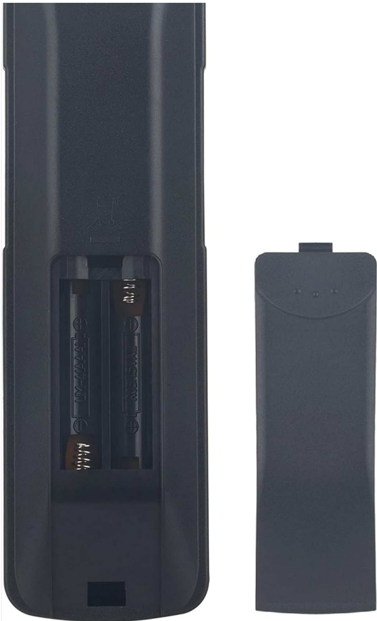
Figure 1: Back of the remote control with the battery compartment open. Insert two AAA batteries as shown, observing polarity.
