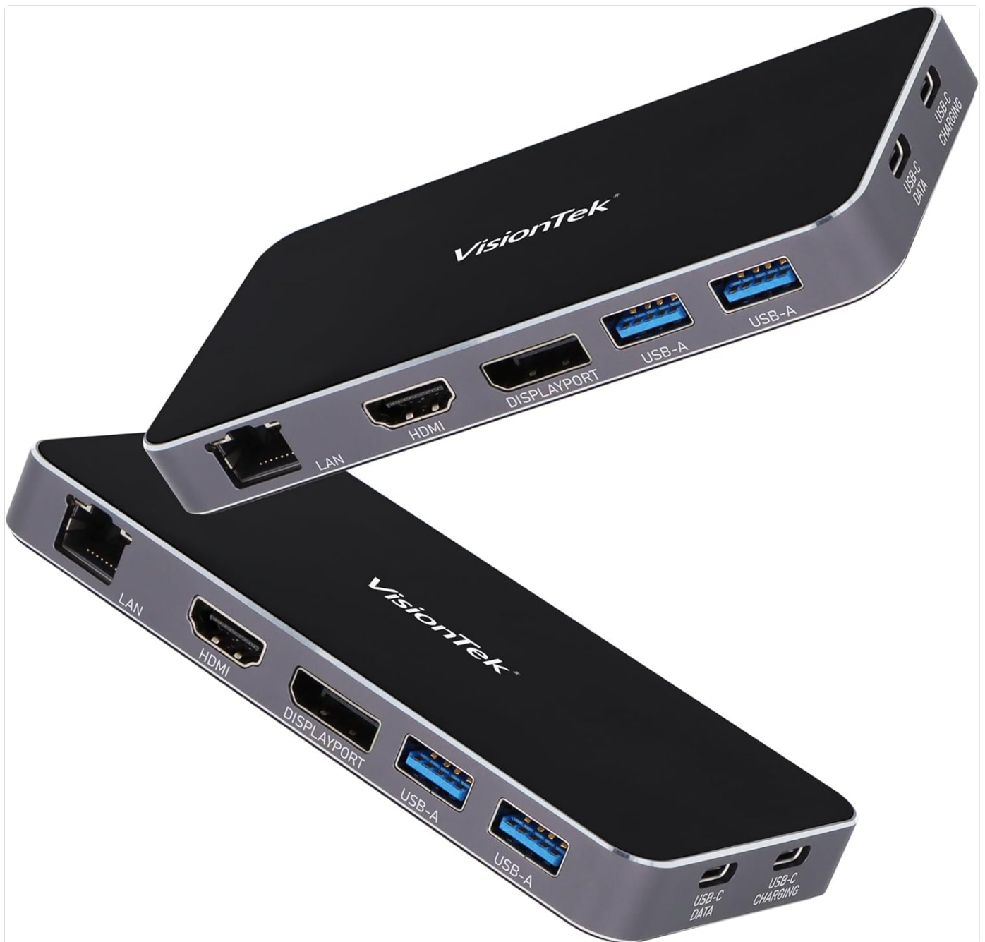
Figure 1: VisionTek VT400 Portable USB-C Dual Monitor Hub, showcasing its compact design and various ports.
