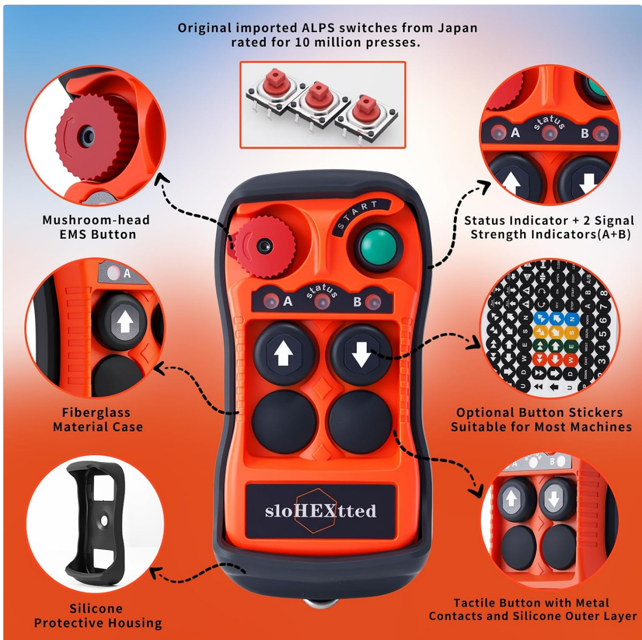
Figure 2.1: Transmitter overview showing mushroom-head EMS button, status indicators, fiberglass case, silicone housing, and tactile buttons.
