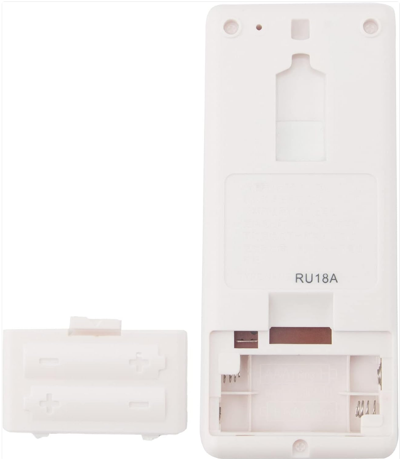
Figure 2: Rear view of the remote control with the battery cover removed, illustrating the battery insertion points. Note the "RU18A" model designation on the back casing.
