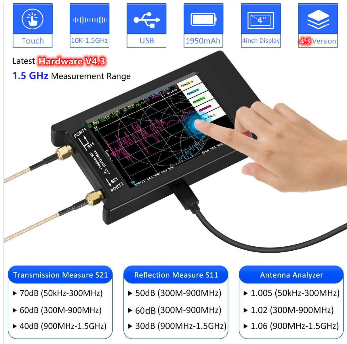
Figure 4.1: The NanoVNA-H4's 4-inch display supports touch input. Key features include 10KHz-1.5GHz frequency range, USB connectivity, 1950mAh battery, and Hardware Version 4.3.
