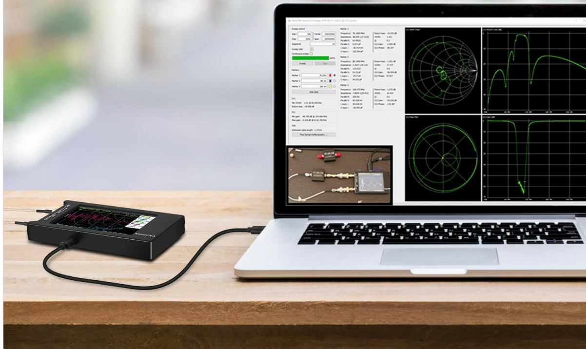
Figure 4.3: The NanoVNA-H4 connected to a PC, displaying measurement data via NanoVNASaver software.
