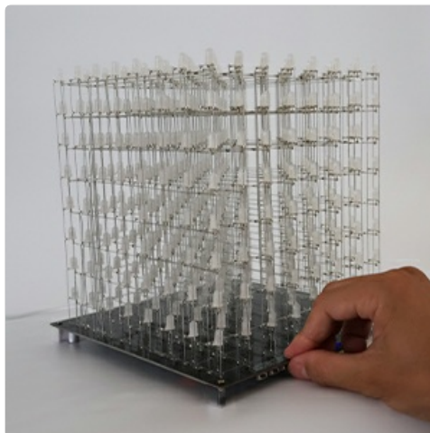
Image: An assembled LED grid being carefully positioned onto the main control board.
