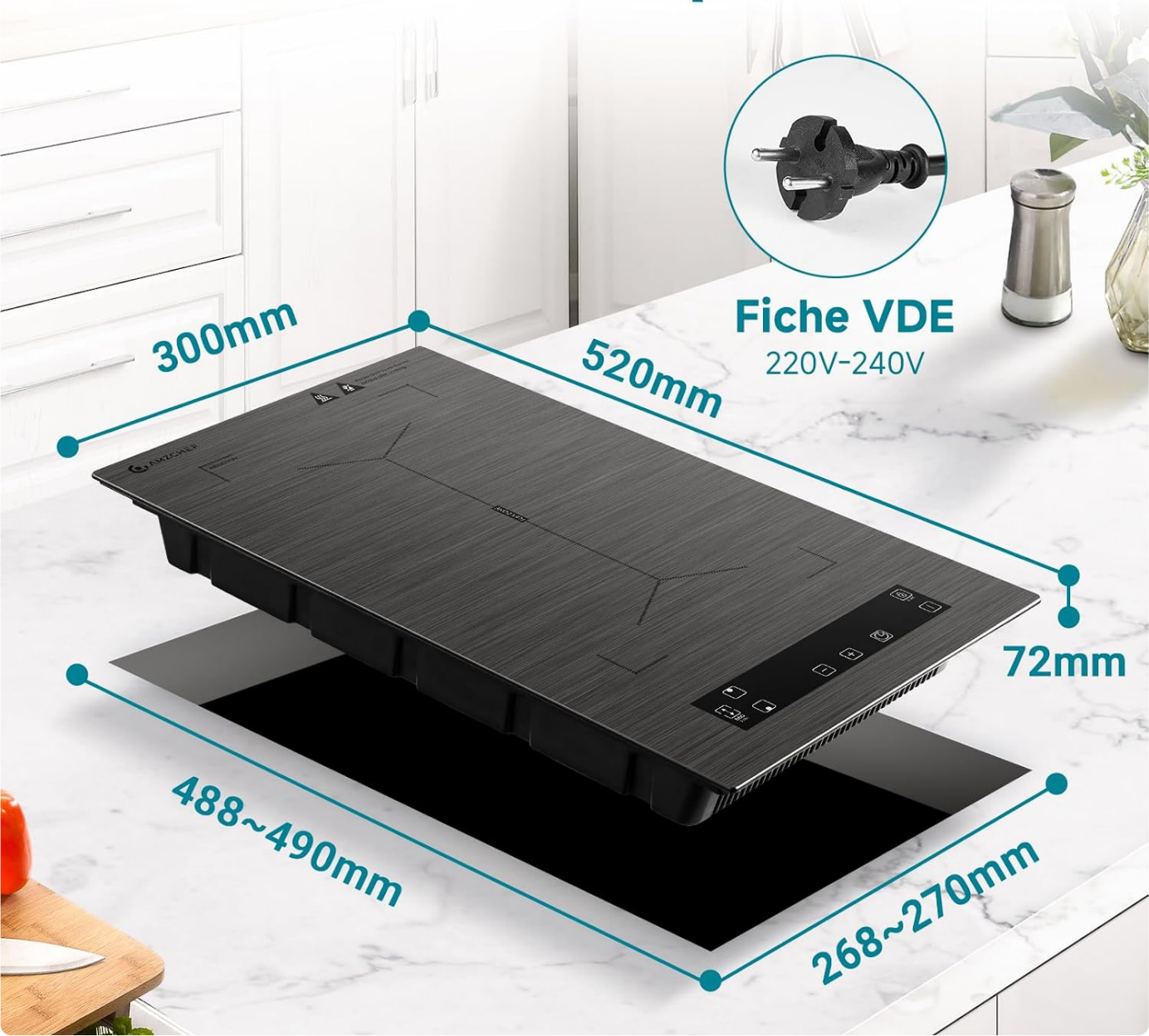
Figure 8.1: Detailed product dimensions and recommended cutout dimensions for built-in installation.
