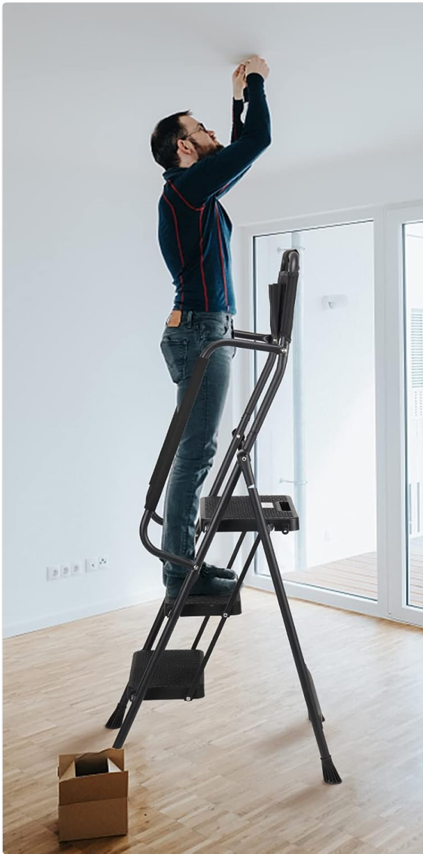
Image 2.1: Illustration of proper contact for the large rubber padded feet to ensure stability and prevent floor scratches.
