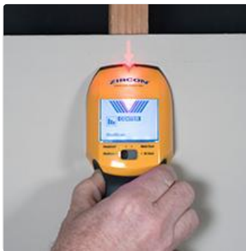
Figure 6: Using Metal Scan mode to detect pipes
