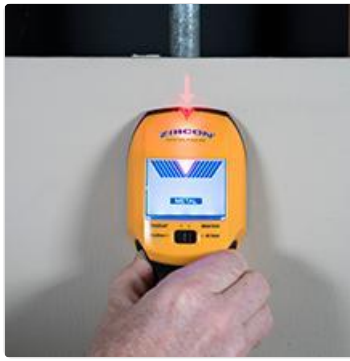
Figure 4: Using StudScan mode to find a stud
