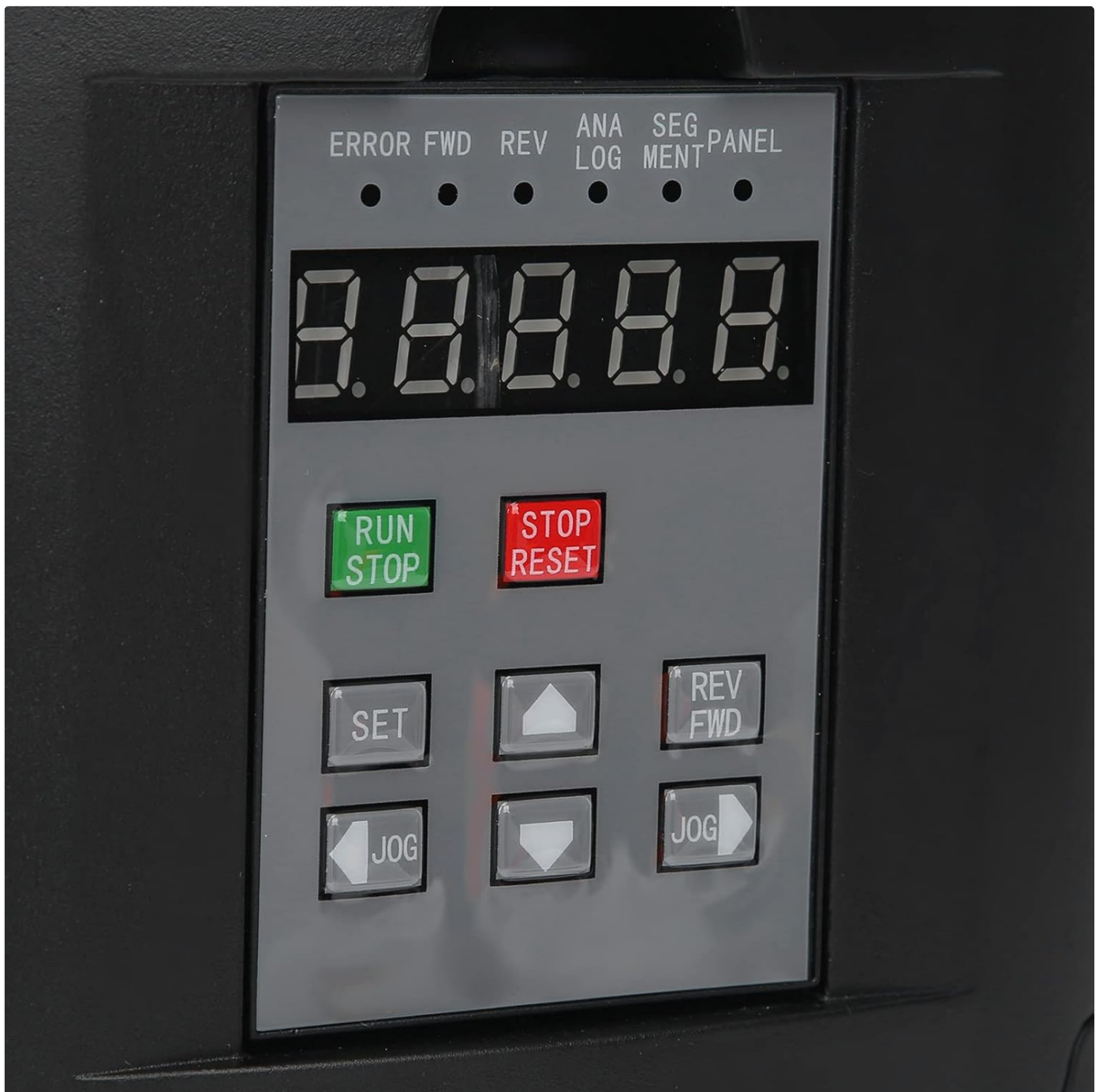
Figure 6: Close-up view of the VFD's control panel, detailing the display and button layout.
