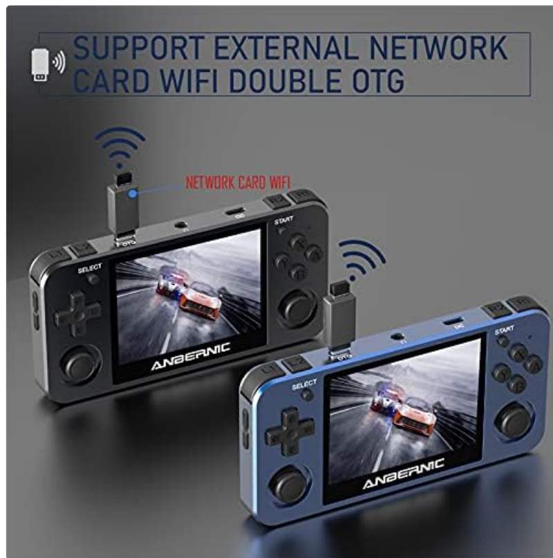
Image 4.5: The RG351MP console demonstrating the connection of an external Wi-Fi dongle for network access.
