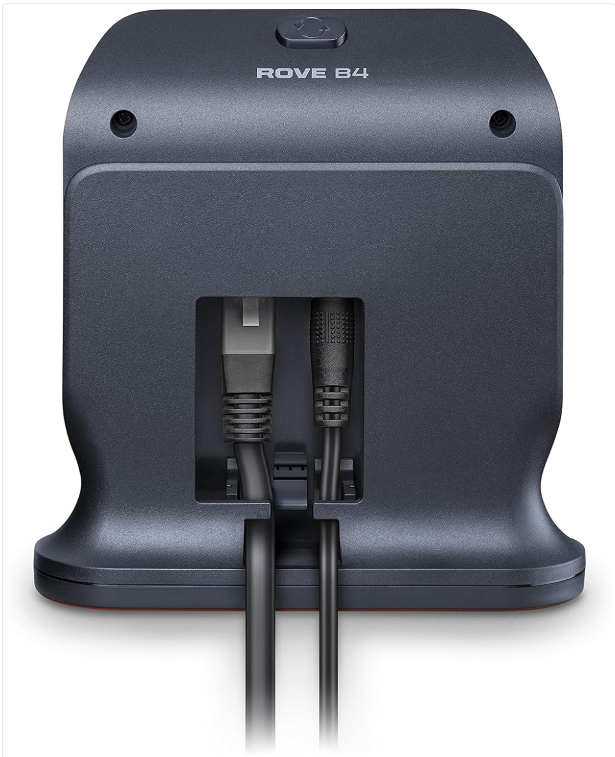
Figure 3.3: Rear view of the Poly Rove B4 Multi-Cell DECT Base Station. This image displays the Ethernet port and power input, with cables connected and routed through the stand for cable management. The model name "ROVE B4" is visible at the top.
