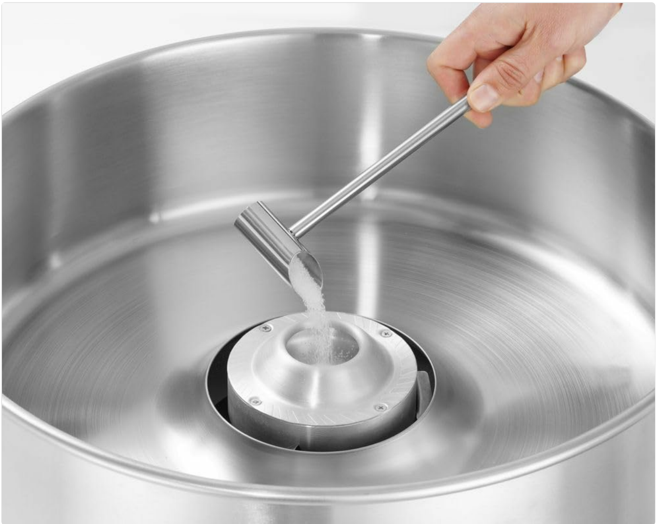
Figure 4.1: Carefully adding cotton candy sugar into the central heating element. Use the provided scoop for precise measurement.
