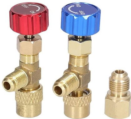
Figure 2: Diagram illustrating the components of the safety valve set. The blue valve is for 1/4 SAE (R22), the red valve is for 5/16 SAE (R410), and the adapter transforms 5/16 SAE to 1/4 SAE.
