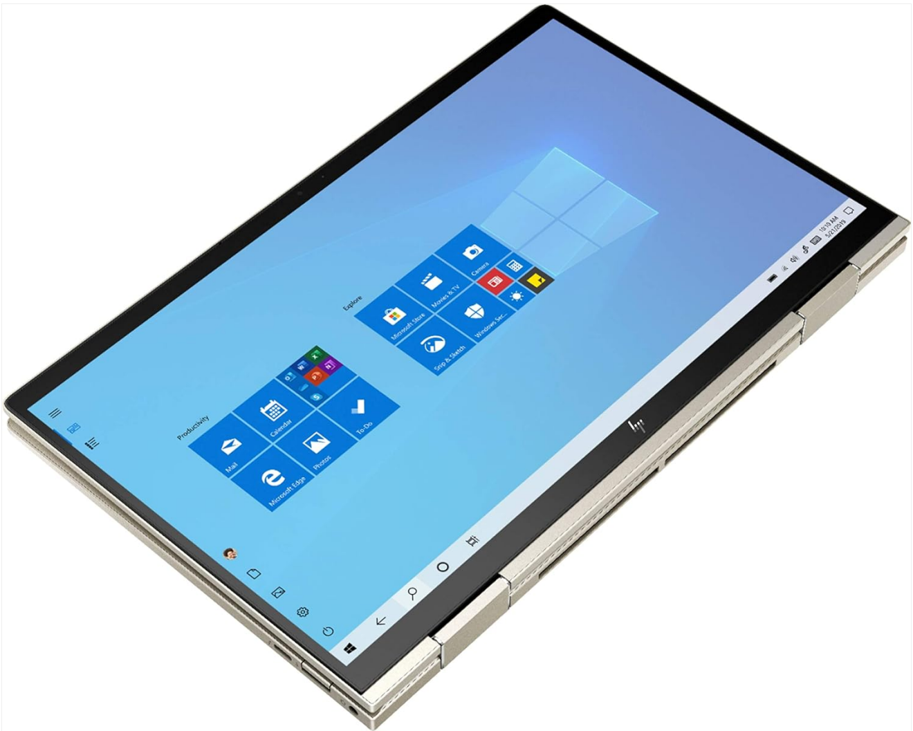
Figure 5.2: The HP Envy x360 laptop fully folded into tablet mode, ready for touch input.
