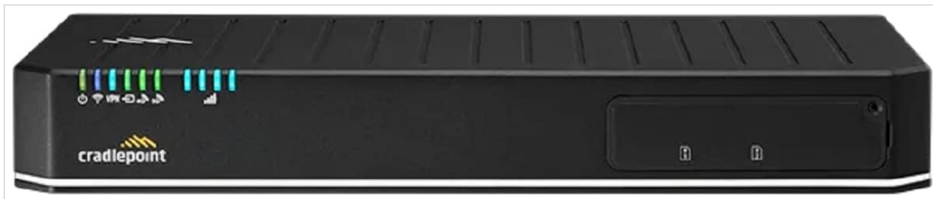
Figure 2.1: Front View of the Cradlepoint E3000 Router. This image displays the front panel of the E3000 router, featuring status indicator lights on the left and two SIM card slots on the right, protected by a cover. The Cradlepoint logo is visible below the indicators.
