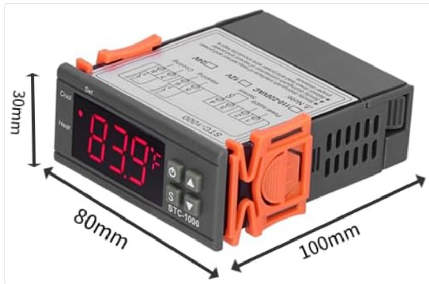
Figure 4.1: Approximate dimensions of the STC-1000 controller.
