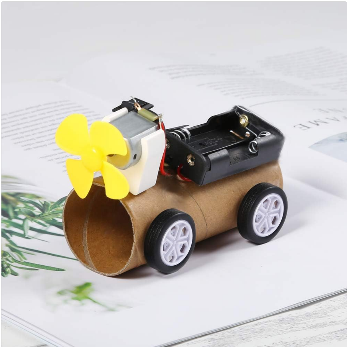
Figure 5: An example of a DIY car project constructed using a DC motor, fan, battery holder, and a cardboard tube.
