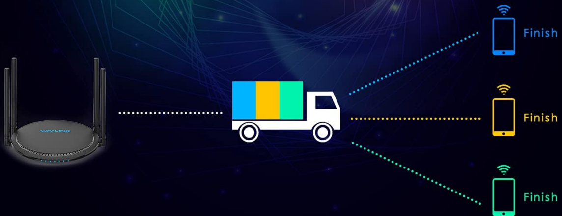
Figure 3.3: Save the Connected Device Battery Life. This image demonstrates how Wi-Fi 6 routers with TWT technology can effectively reduce the power consumption of terminal equipment compared to Wi-Fi 5 routers.
