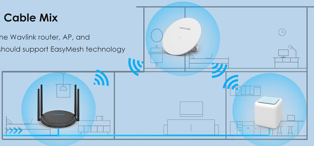
Figure 3.4: Mesh Networking. This diagram illustrates various mesh networking configurations: via cable, via wireless, and a wireless & cable mix, enabling seamless and easy network creation.
