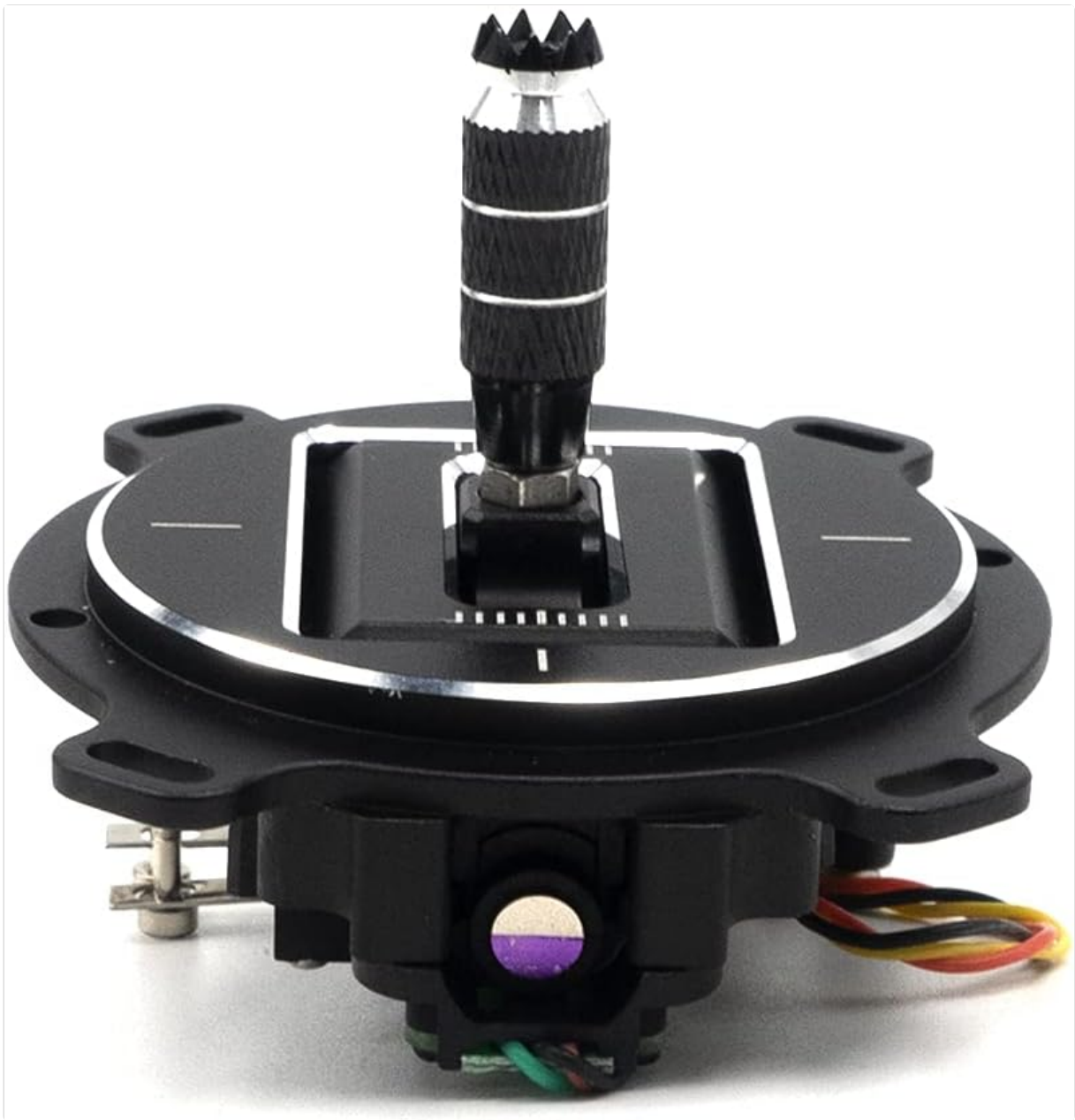
Figure 4.1: Front view of the MC11 Gimbal with the control stick.
