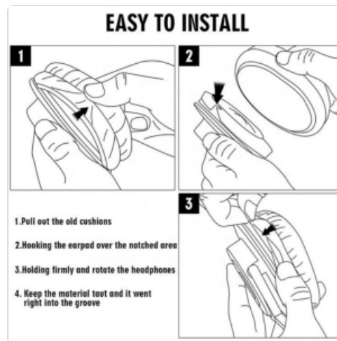
Image 3: Diagram illustrating the four steps for installing replacement earpads onto headphones.
