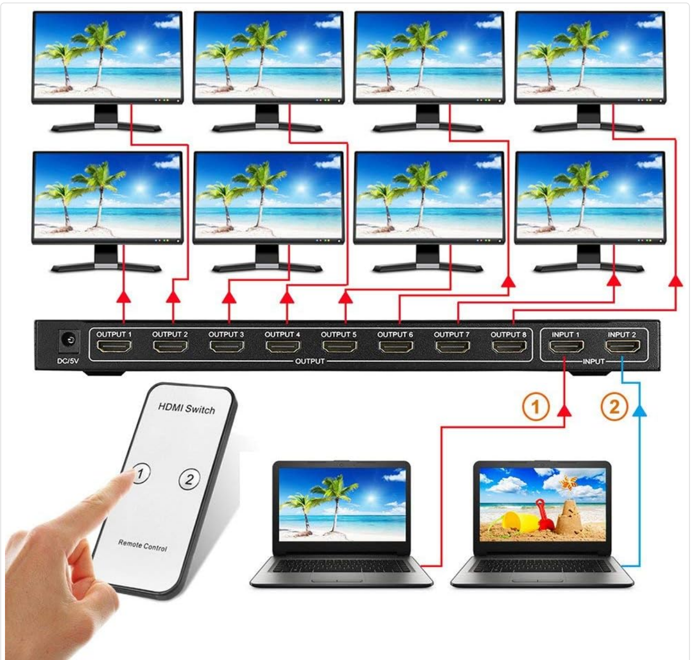
Image: An alternative connection diagram demonstrating two laptops as input sources feeding into the splitter, which then distributes the signal to eight separate monitors. The remote control is also depicted, indicating its role in input selection.
