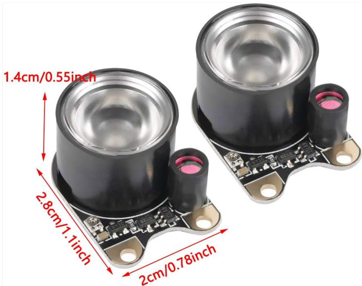
Figure 4.2: Dimensions of the LED fill light module: 2.8cm (1.1 inches) in length, 2cm (0.78 inches) in width, and 1.4cm (0.55 inches) in height.
