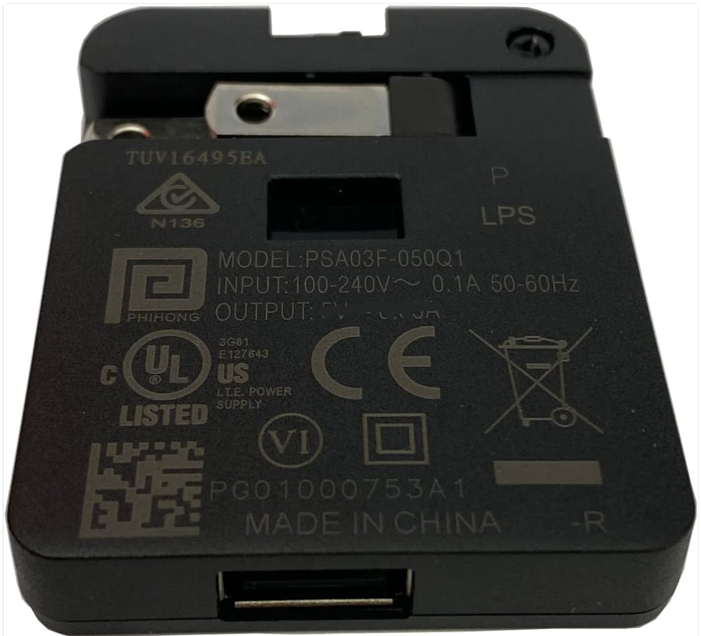
Image: The UpBright AC/DC adapter, displaying its model number, input (100-240V, 0.1A, 50-60Hz), and output (5V) specifications, along with safety certifications.
