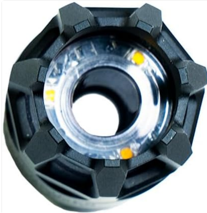
Figure 6: Front view showing the LED array.
