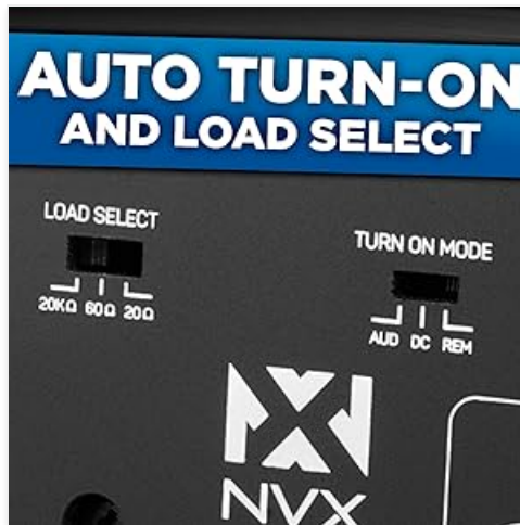
Figure 4.3: Auto Turn-On and Load Select Switches.
