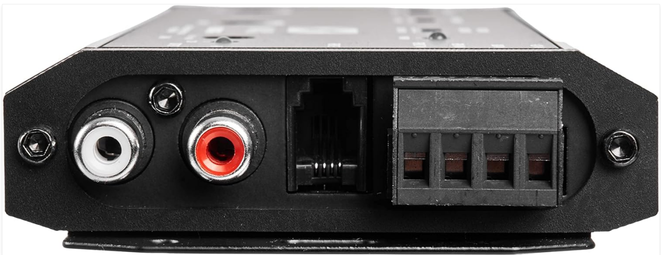
Figure 5.3: RCA Output and Remote Port.
