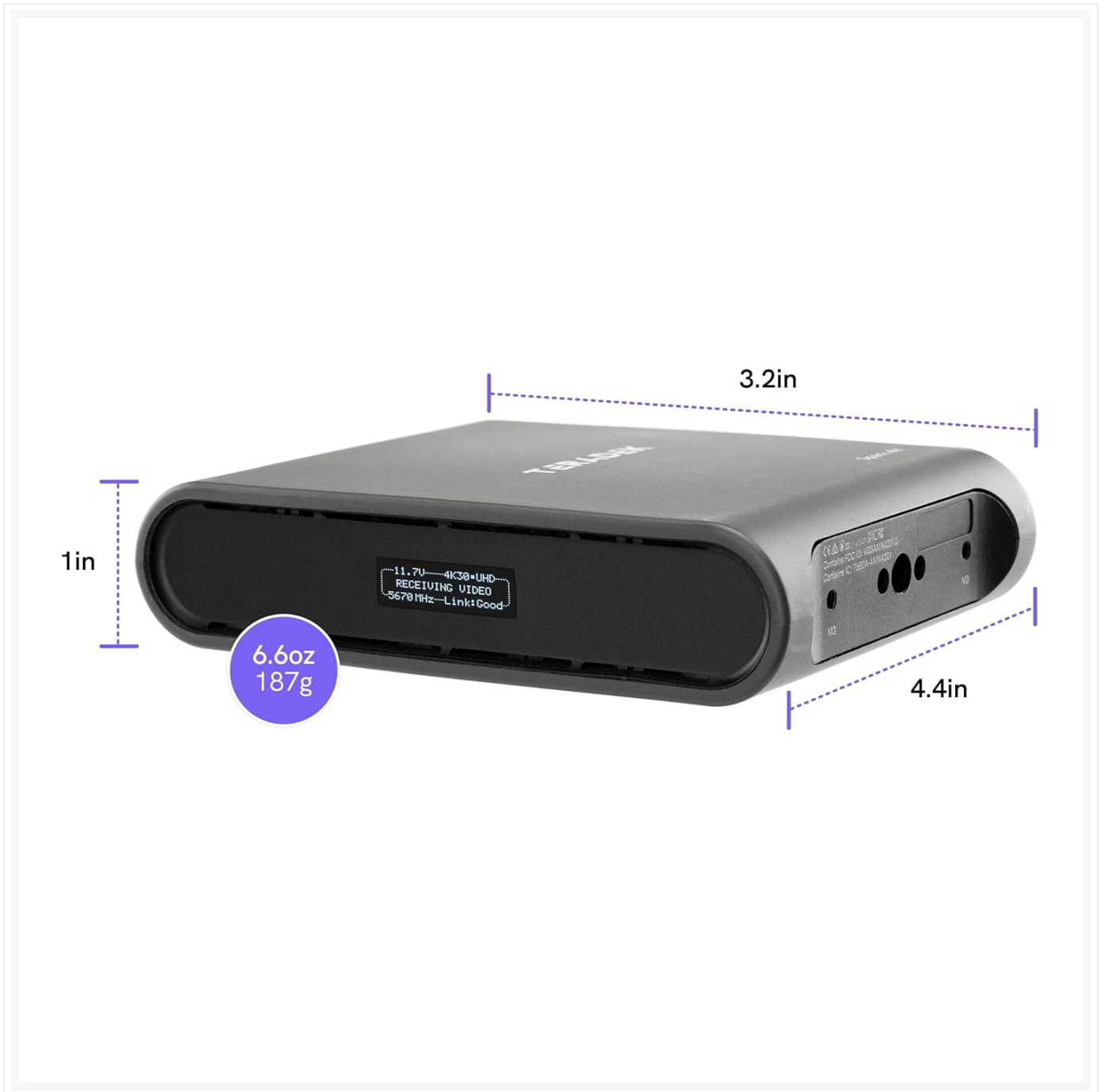
Figure 4.1: Dimensions and weight of the Spark 4K Receiver.
