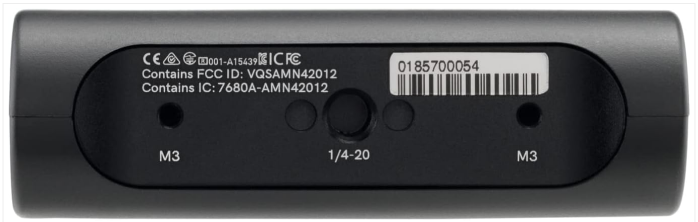
Figure 4.3: Bottom of the Spark 4K Receiver with mounting options.
