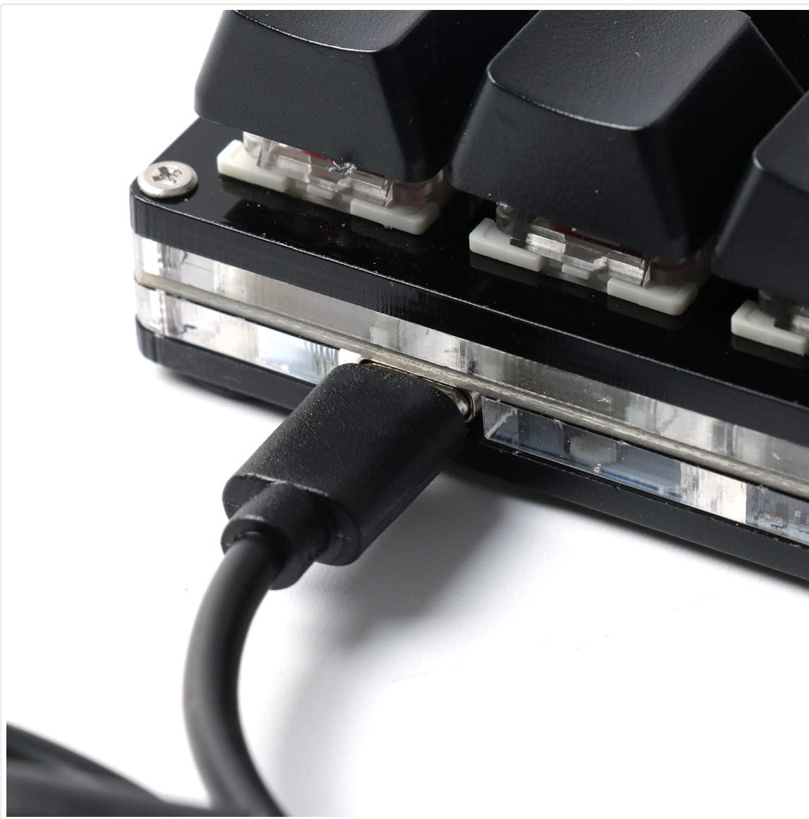
Image: Close-up view of the USB-C port on the side of the keyboard with the cable inserted.
