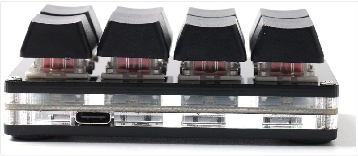
Image: Side view of the keyboard, revealing the mechanical switches beneath the keycaps.
