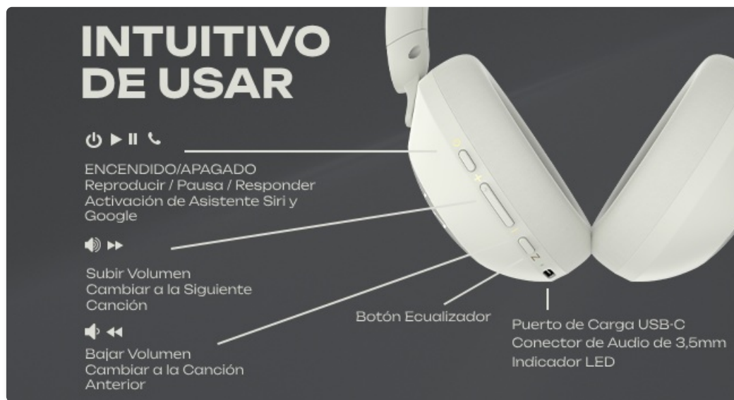
Image: An illustration detailing the control buttons and ports on the PowerLocus Orion headphones. It shows the Power On/Off, Play/Pause/Answer Call, Siri/Google Assistant activation, Volume Up/Next Song, Volume Down/Previous Song, EQ Button, USB-C Charging Port, and LED Indicator.
