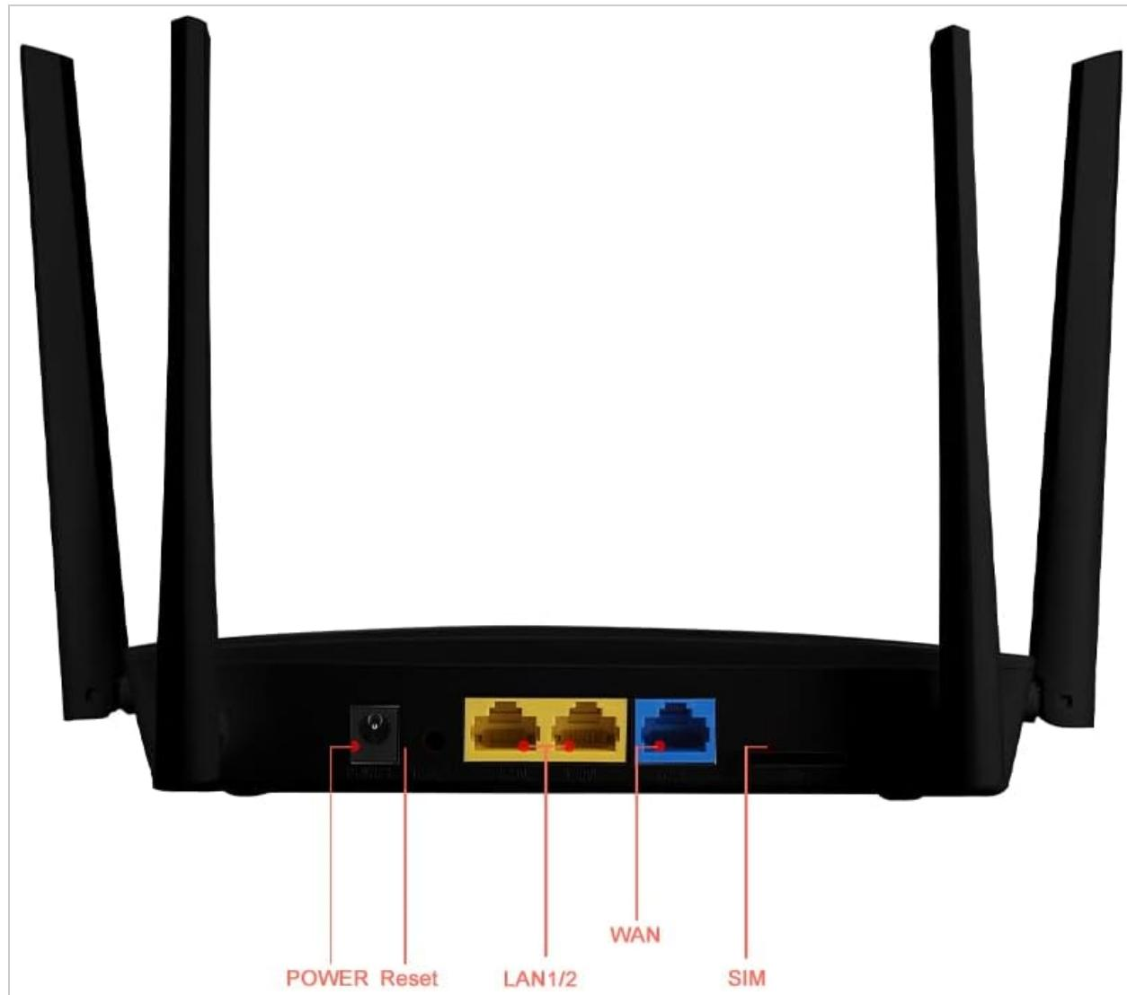
The rear panel of the router features the power input, a reset button, two LAN ports for wired connections, a WAN port for external internet connection, and the dedicated slot for inserting the SIM card.
