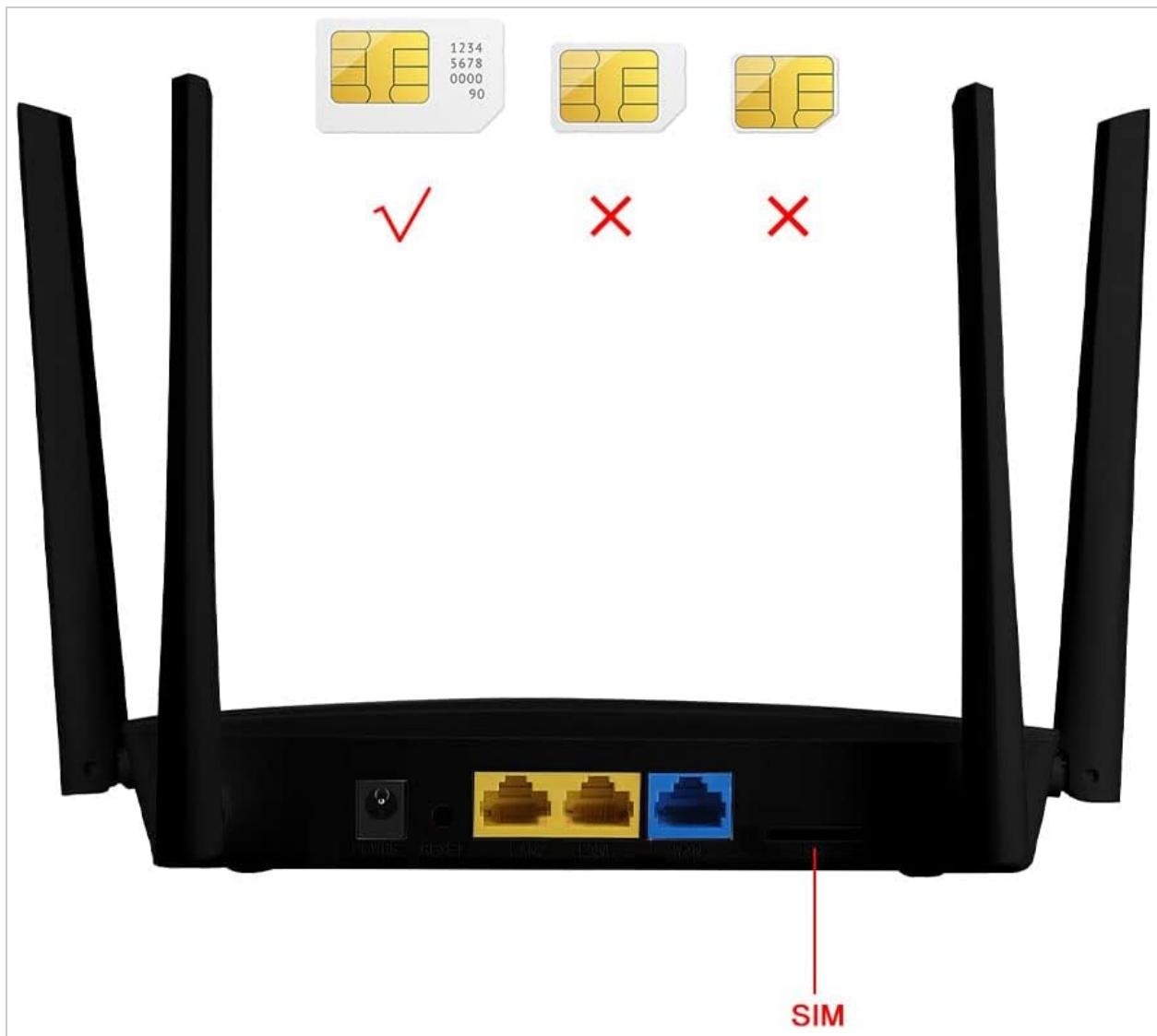
This image illustrates the compatible SIM card size for the router. Only standard-sized SIM cards are supported. Micro and Nano SIM cards are not compatible and should not be used directly without an adapter.
