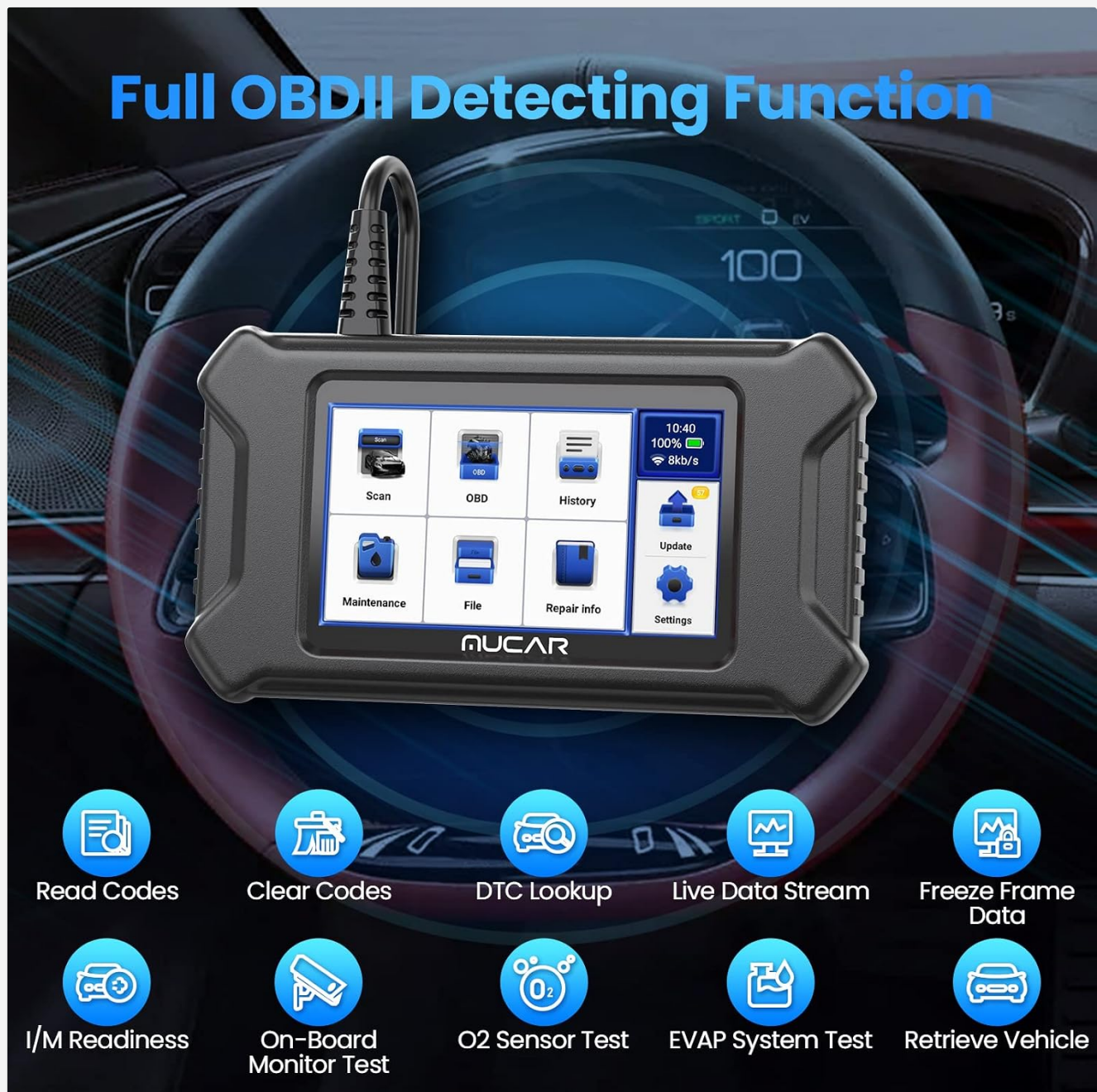
Image 4.4: The MUCAR CS99's comprehensive suite of OBDII diagnostic functions.
