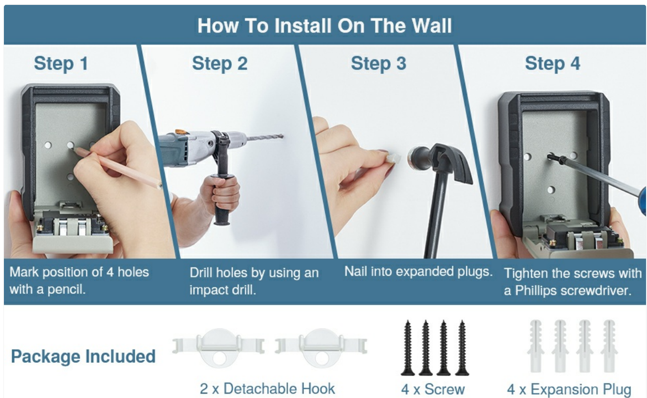
Image 3.1: Step-by-step guide for wall mounting the key lock box.
