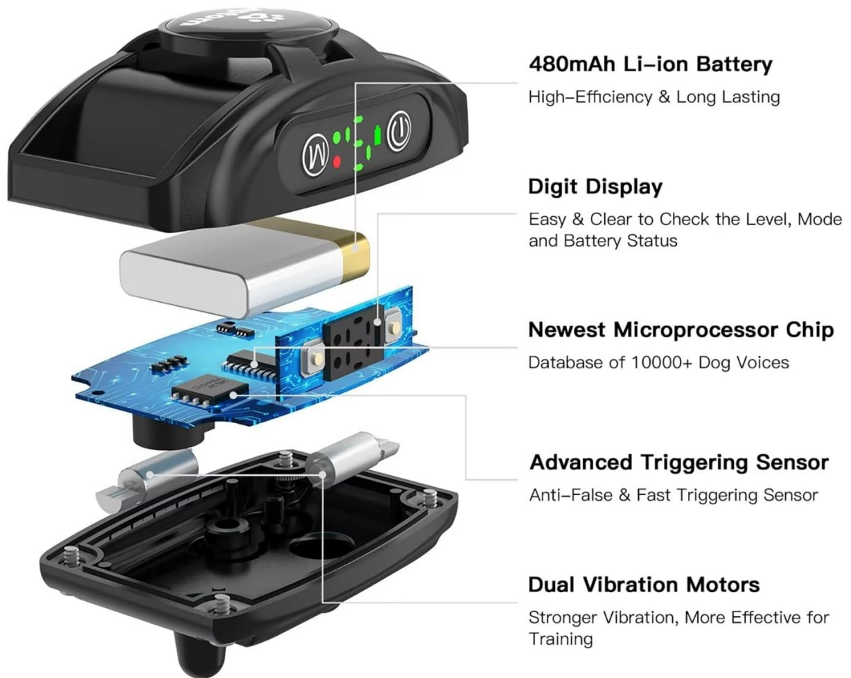
Figure 4: Collar Unit Overview with Labeled Components
