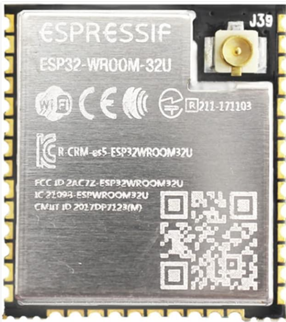
Figure 2: Detailed view of an ESP-WROOM-32U module. The image clearly shows the U.FL connector, various regulatory marks (Wi-Fi, CE, FCC ID), and a QR code.
