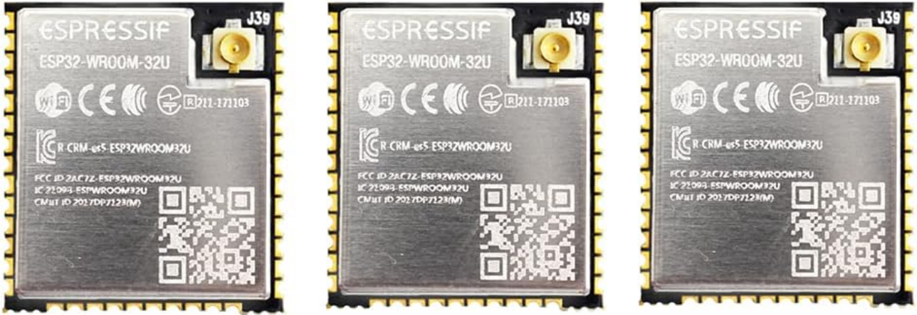
Figure 1: Overview of multiple ESP-WROOM-32U modules. Each module features an Espressif logo, Wi-Fi and CE markings, and a U.FL connector for an external antenna.
