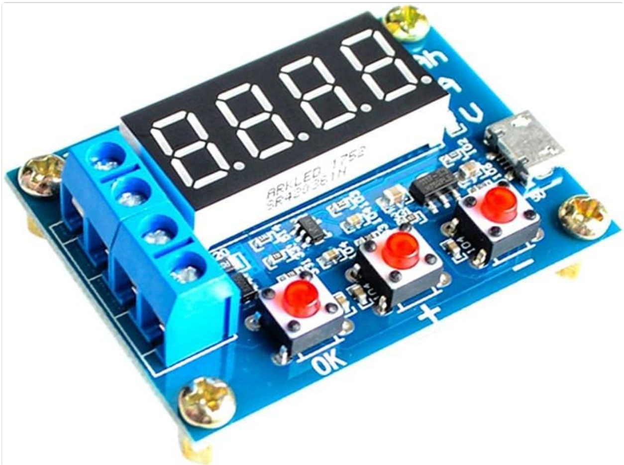
Figure 1: ZB2L3 Battery Capacity Tester showing the micro USB power input, battery terminals, and load terminals.
