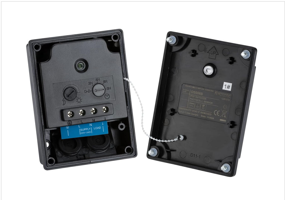
Figure 2: Internal view of the OS006B switch. The left side shows the circuit board with terminals labeled L, N, and LOAD, along with dials for adjusting light sensitivity and timer settings (2H, 4H, 6H, 8H, D-D). The right side shows the inside of the cover with product information.
