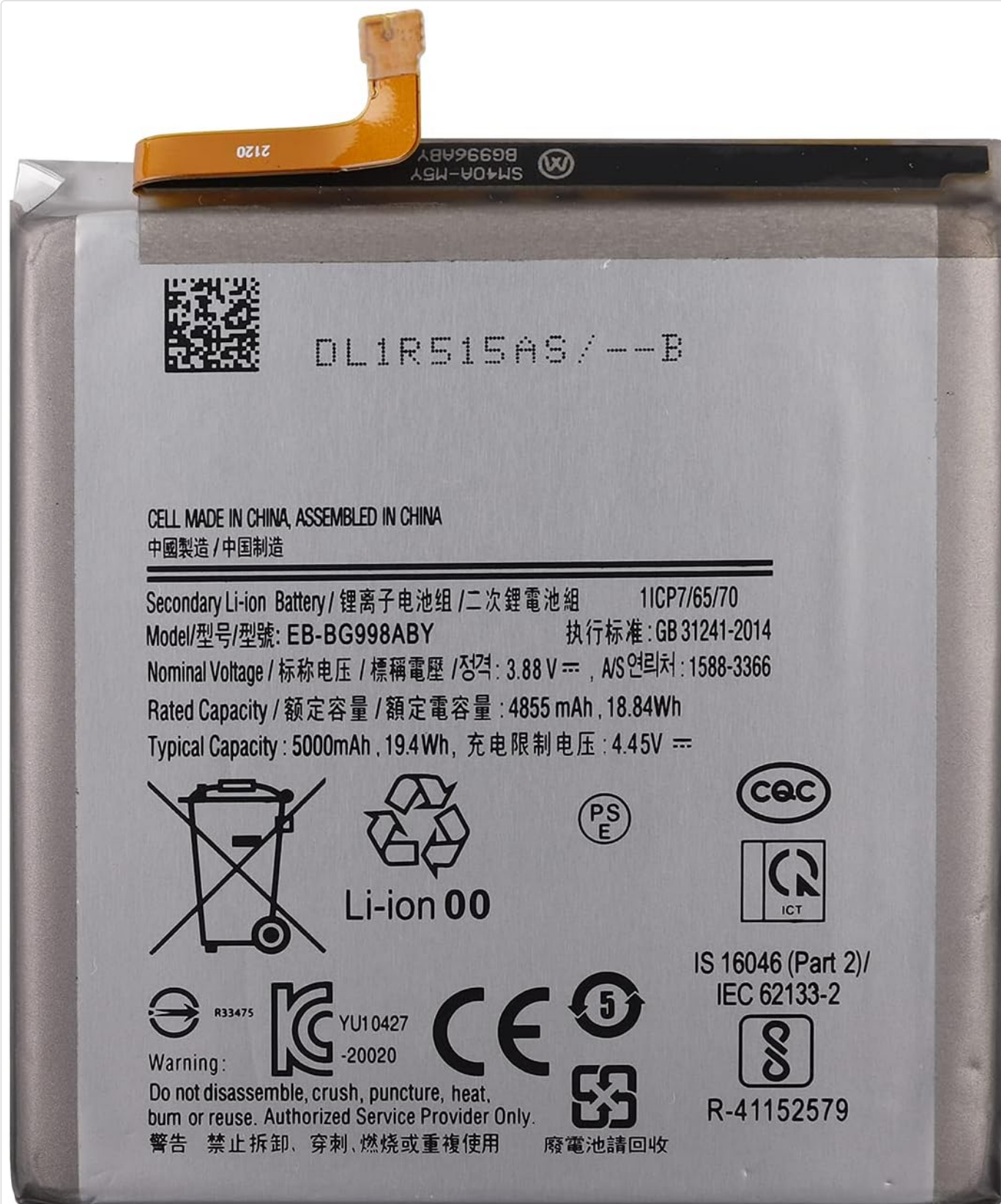
Image 4: Detailed view of the Duotipa EB-BG998ABY battery's front, displaying its model number and technical specifications.
