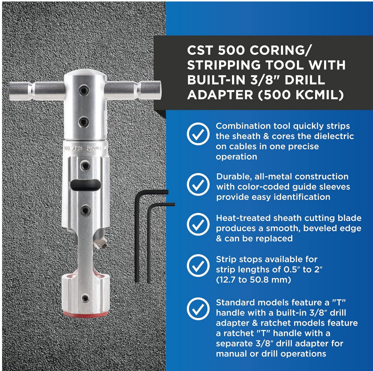
Image 3.2: Visual representation of the CST 500's primary features, including its combination stripping and coring function, durable construction, and replaceable blades.
