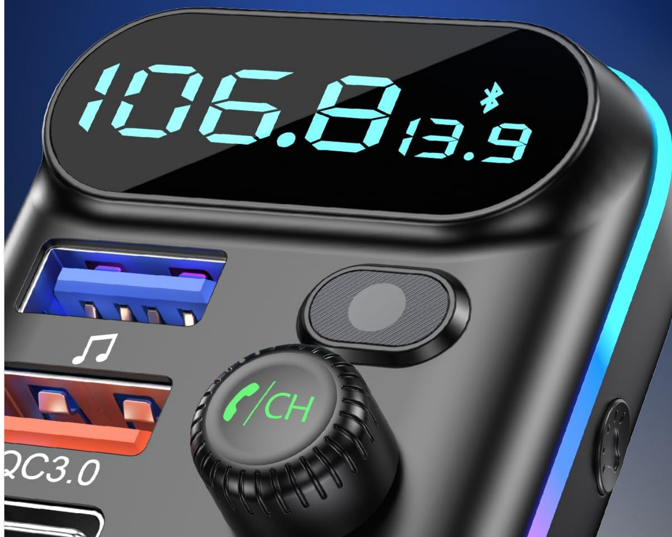
Image 4.1: Close-up of the LENCENT FM Transmitter's LED display, showing Bluetooth connection, FM station number, and car voltage indicators.
