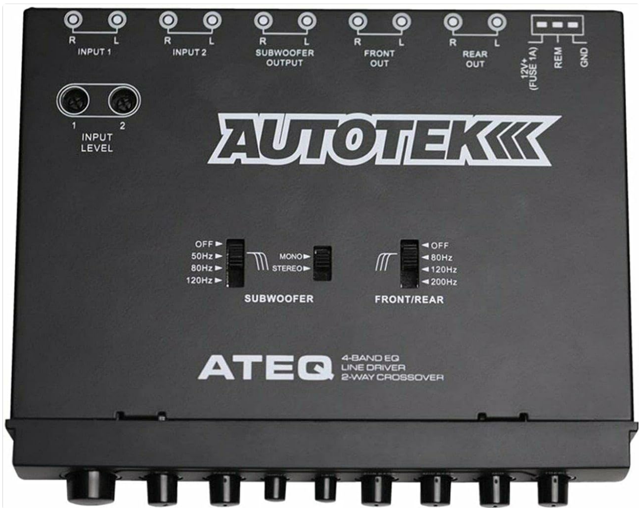
A detailed top-down view of the Autotek ATEQ PK1 equalizer, highlighting the RCA input jacks (Input 1, Input 2), subwoofer output, front and rear outputs, power connections (12V+, REM, GND), input level controls, and the selectable switches for subwoofer crossover frequency (OFF, 50Hz, 80Hz, 120Hz), mono/stereo subwoofer mode, and front/rear high-pass crossover frequency (OFF, 80Hz, 120Hz, 200Hz).
