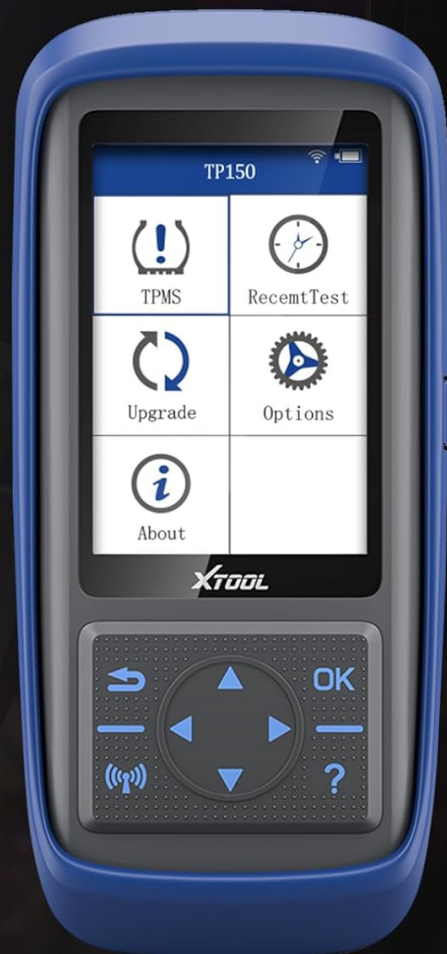
Figure 3.4: TPMS diagnosis interface on the XTOOL TP150, showing options to read/clear codes and turn off warning lights.
