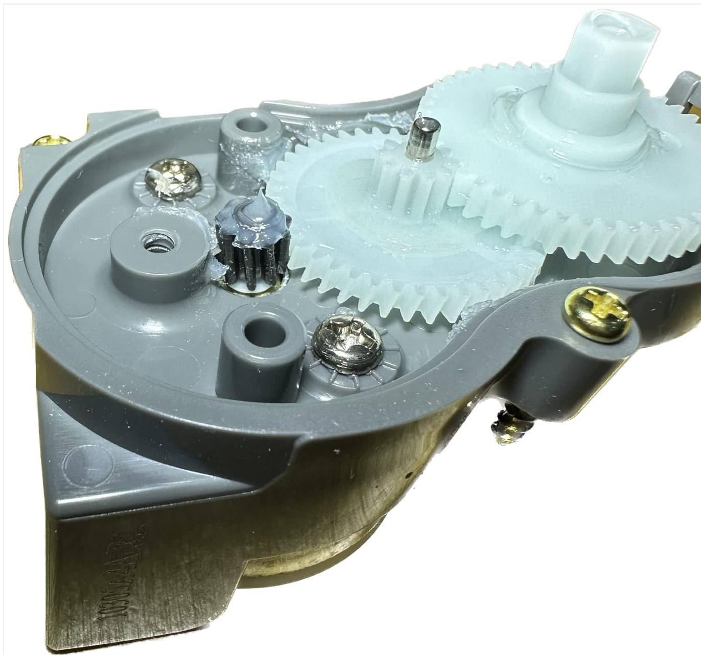
Figure 2: Internal view of the module, highlighting the improved spiral gear teeth designed for enhanced durability.
