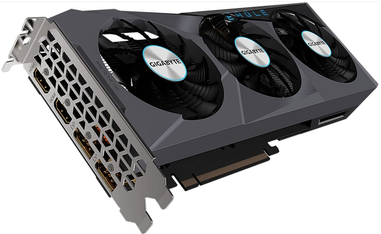
Figure 2.1: Front view of the GIGABYTE Radeon RX 6600 XT Eagle 8G Graphics Card, showcasing the WINDFORCE 3X cooling system with three fans.
