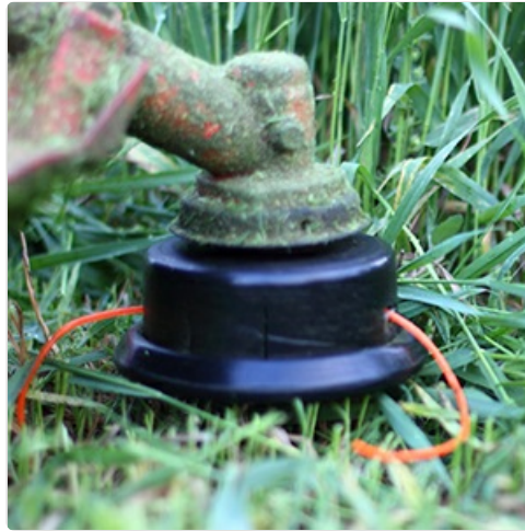
Image 7.1: A detailed view of the trimmer line properly fed through the eyelet of the trimmer head.
