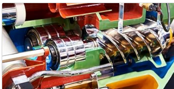
Image 4.2: An internal view of a compressor mechanism, illustrating the components that benefit from proper lubrication.
